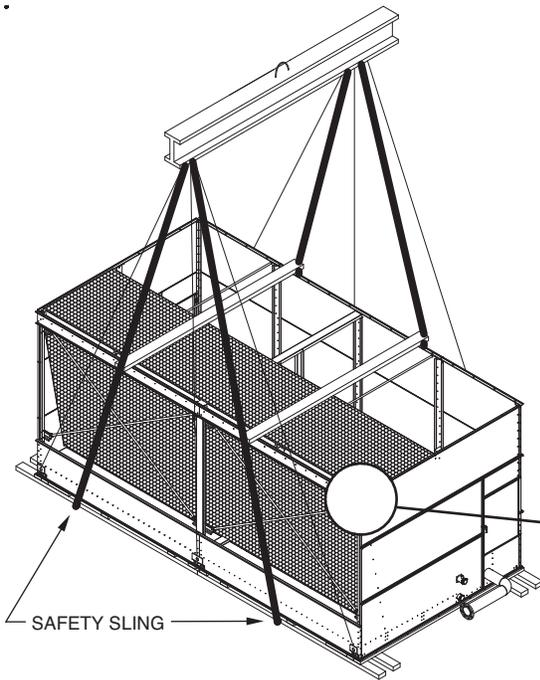
Figure 6 – Proper Rigging Method for Extended Lifts
