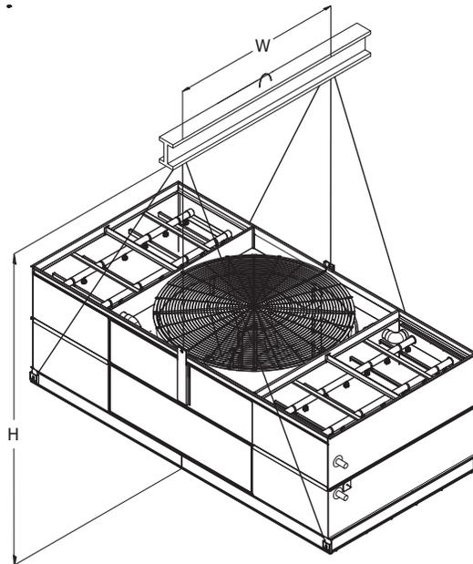
Figure 11 – D Model Coil / Fan Section – 24' and 26' Long
