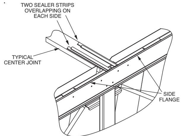
Figure 8 – Sealer Detail for Center End Flange Joint of S and L Models with 18' or 24' Coil Sections
