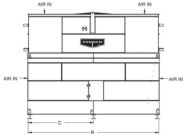
Figure 2 – Recommended Steel Support for D Models
