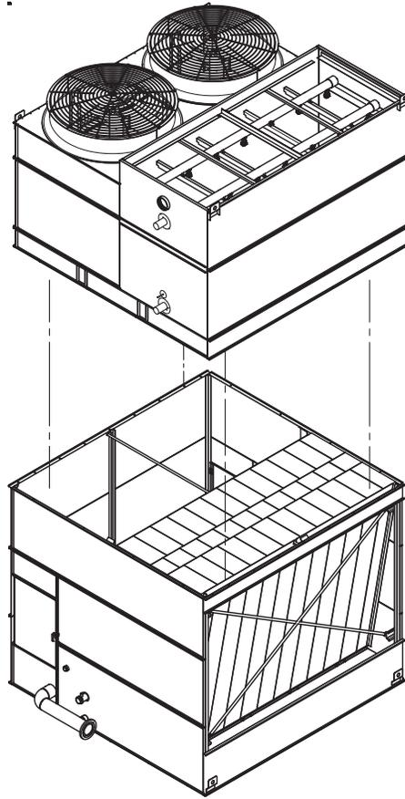
Figure 12 – Mating Upper Coil / Fan Section to Basin Section
