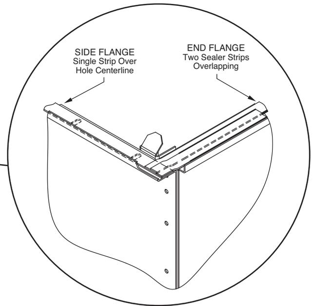
Figure 7 – Proper Sealer Tape Application
