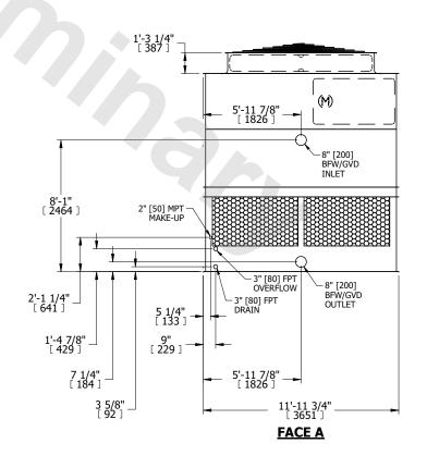
NO. OF SHIPPING SECTIONS **SHIPPING** OPERATING HEAVIEST SECTION 6740 lbs+ [3060] kg+ 11700 lbs+ [5310] kg+ 4320 lbs+ [1960] kg+ WEIGHT WEIGHT WEIGHT
