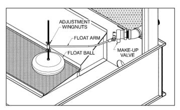
Figure 13 - Mechanical Water Make Up Valve
