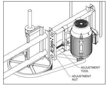
Figure 5 – AT Motor Adjustment
