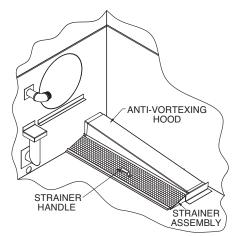
Figure 10 - LSTE/PMTQ Strainer Assembly
