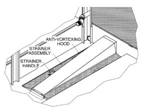
Figure 9 – Dual Strainer Assembly
