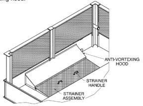
Figure 8 – Single Strainer Assembly
