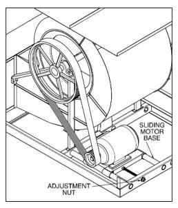
Figure 7 – LPT Motor Adjustment
