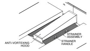
Figure 12 - AXS Strainer Assembly
