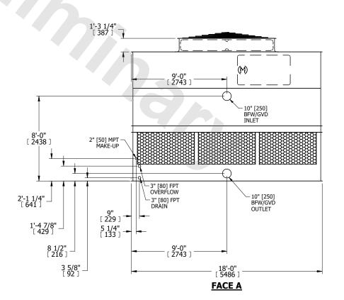
DRAWN BY: KDS NO. OF SHIPPING SECTIONS **SHIPPING** OPERATING HEAVIEST SECTION 9190 lbs+ [4170] kg+ 16790 lbs+ [7620] kg+ 5640 lbs+ [2560] kg+ WEIGHT WEIGHT WEIGHT
